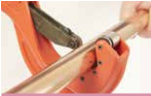
1. Cut the tube to length
