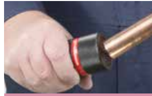
2. Deburr and remove all external sharp edges
