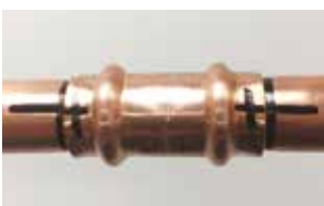
11. Mark the completed joint
